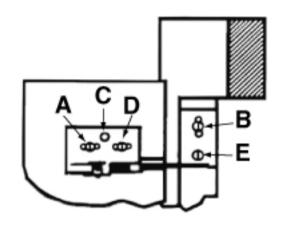
Install hinges on door using screw slot (A) or (D). Install all doors on cabinet using only screw (B) - then adjust all doors for fit. Then install the remaining screw in (E) on the stile and in (C) or the remaining adjustment slot on the door. (Recommended minimum face frame size is 1-1/2 inches)
