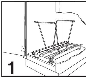
With the frame in a closed position, insert the front two screws, making sure that the framework is square to the front of the cabinet.
