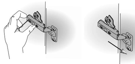
Press button on rear of hinge arm.
