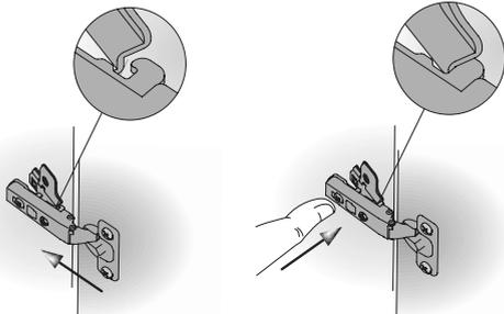
Slide two hooks under hinge arm into the mounting plate.
