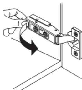
Release the lever under the hinge arm to remove.
