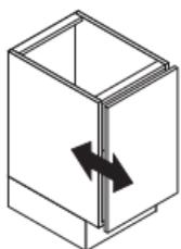
Rotate back screw to adjust door position.
