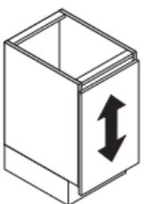
Rotate cam screw to adjust door height up or down.
