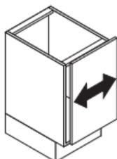
Turn front screw clockwise to increase door overlay, counter-clockwise to decrease.
