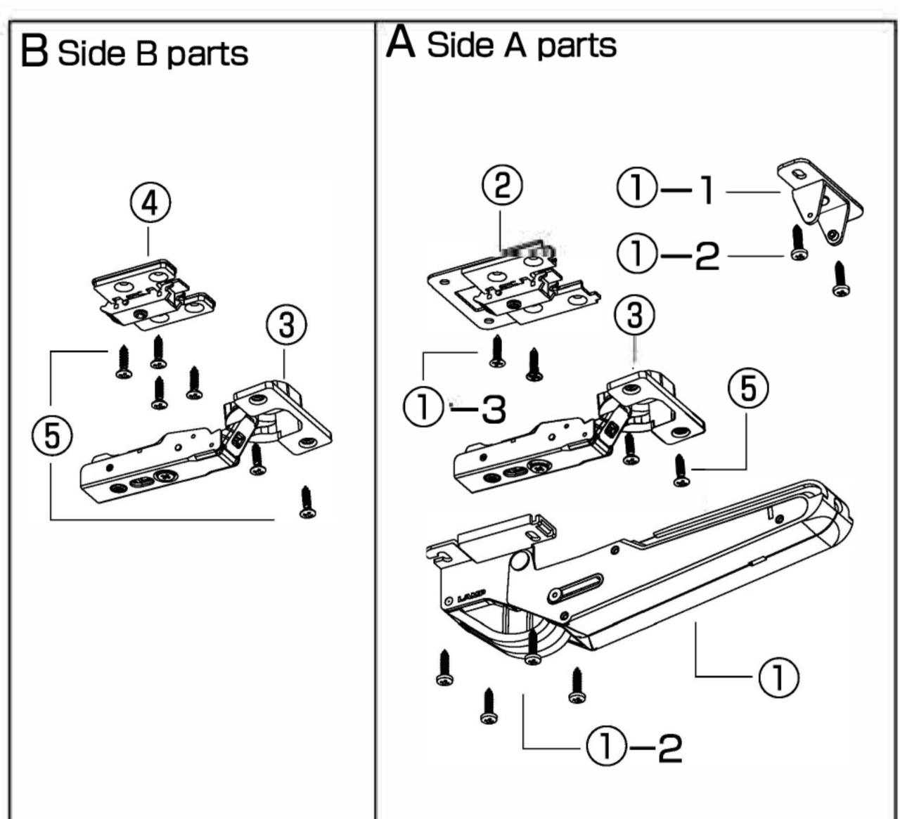
The quantities of parts shown above are an example of a typical installation.
