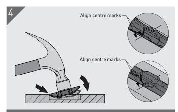
To aid in the installation of the Key and Hook, start by inserting one end in the slot when use a hammer or mallet to tap the component into place. Ensure centre lines on substrate align with centre marks on Hook and Key.
