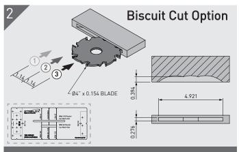
Set the depth stop to #20 and guide height for substrate thickness. Plunge in 3 locations then repeat using the **Mark-Out Template**, packing the guide to achieve a 0.276" cut.
