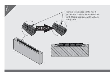
Before assembling the Striplox Mini 120, make note of the locking tab on the Key. Leaving this tab in place will prevent the unintentional unlocking of the joint.
