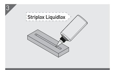
Apply Striplox Liquidlox 15 second cure adhesive to both sides of the slot in each substrate. *Visit joinlox.com/striplox or call 1800 JOINLOX to find out more about Striplox Liquidlox and Mark-Out Template.*
