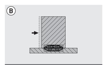
To complete the assembly push the end of the substrate (with X offset) until the Mini 60 is fully engaged.
