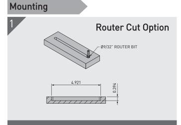
Use a Ø9/32" router bit to cut a slot in both substrates where the Hook and Key of the Mini 120 is to be mounted. Depth needs to be 0.394" for each.
