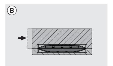
To complete the assembly push the end of the substrate (with X offset) until the Mini 120 is fully engaged.
