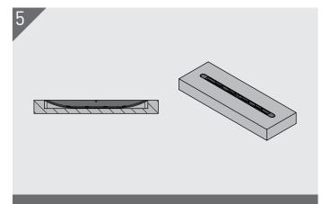
After glue is applied, insert Hook and Key into slot until flush with substrate. Allow to dry as per glue manufactures instructions.
