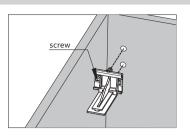
Inset slide end into rear bracket and fix the slide onto the cabinet
