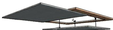
Release 1 panelsafe to hinge panel down
