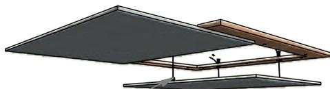
Release 1 panelsafe to hinge panel down
