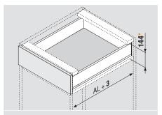
AL = Actual cabinet profile length \*Minimum opening height based on 3 (1/8") clearance
