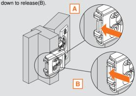
Step 2: While the CLIP lever is released, pull forward on hinge / door to remove from cabinet.
