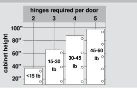
NOTE: The distance between the top and bottom hinges must be greater than the width of the door
