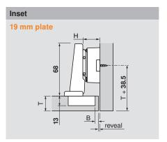
NOTE: With our new CLIP wing mounting plate program, all three of the common frameless applications, (full overlay, half overlay and inset) can be achieved with a straight-arm hinge and cam height adjustment. An alternative inset application, includes the use of a half-cranked hinge and 9 mm cam height adjustment mounting plate.
